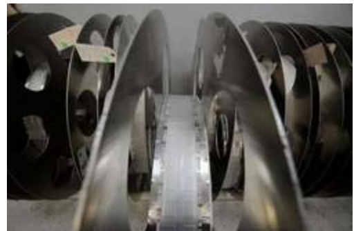
PIERRE DUCHARM | The Ledger Lakeland-based Solicore makes thin, flexible batteries, shown here stored on rolls, that power RFID applications.
